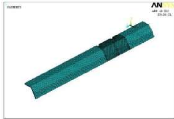
Fig.3.1.meshed element of the HH10 tie.
